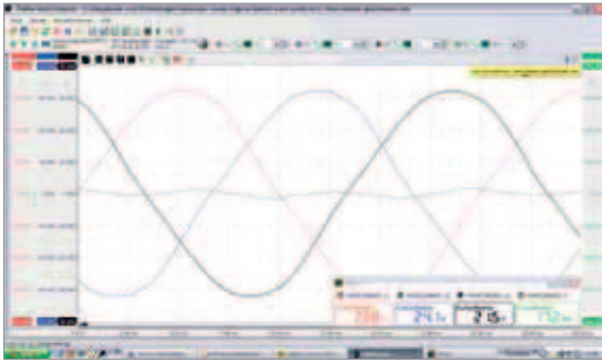
unsymmetrical load, I1 low-resistance, neutral conductor closed
