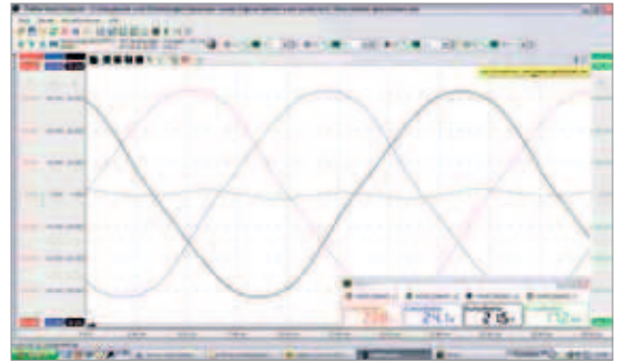
symmetrical load, neutral conductor closed
