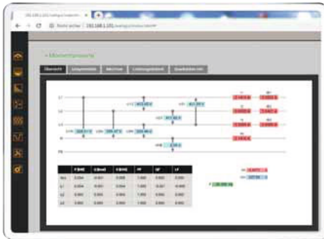
Display of the instantaneous values of current, voltage, power
