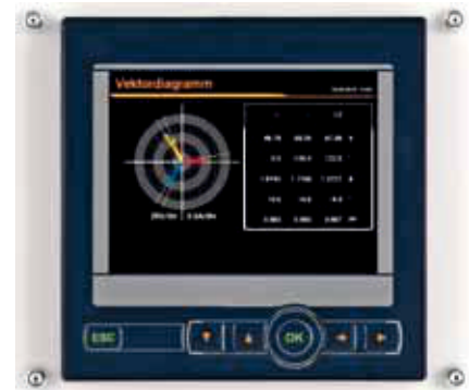
Display of the vector diagram of an inductive consumer, e.g. fluorescent lamp
