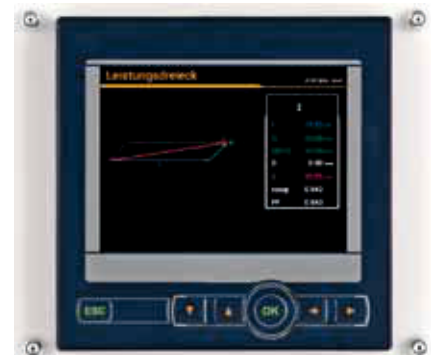
Display of the performance triangle in case of a consumer with harmonics
