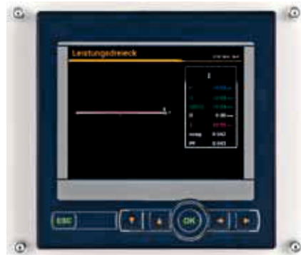
Display of the performance triangle in case of a linear consumer
