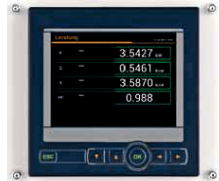
Display of the instantaneous values of current, voltage, power
