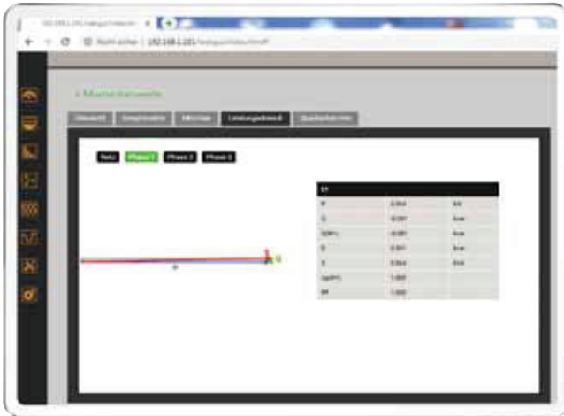
Display of the performance triangle in case of a linear consumer
